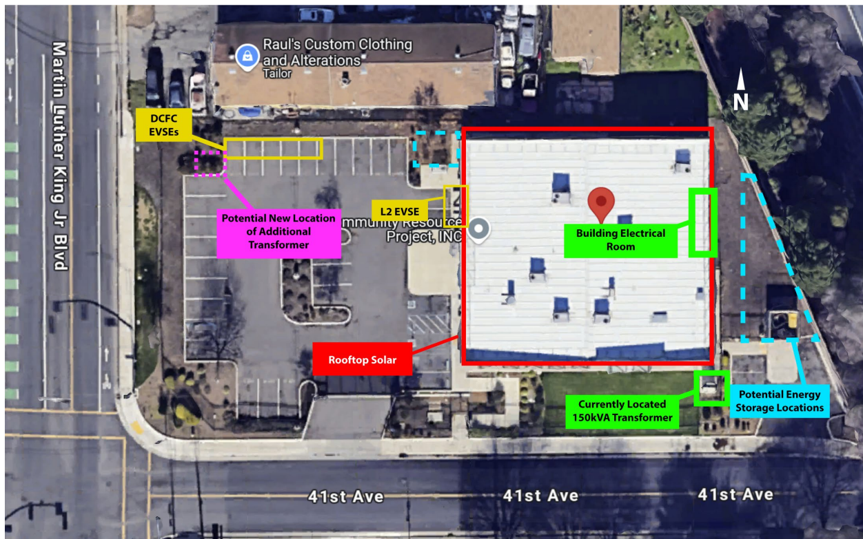
Figure 1 - Site aerial view. Location of chargers, energy storage, or new transformers is not finalized. Current transformer may be replaced with higher capacity rather than adding another one to the site.
